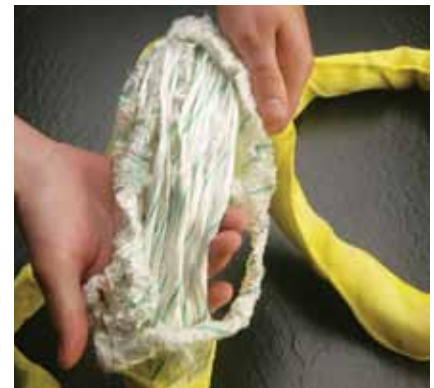
Sling Overload Failure
