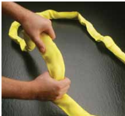
Cover in Good Condition
