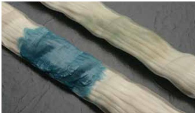
Before and after cleanup of wheel bearing grease.
