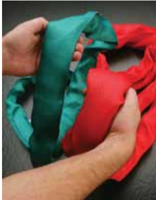
This green roundsling is rated at less than half the capacity of the red.
